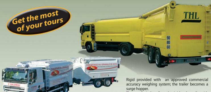
The transfer is done from the rigid to the trailer with an articulated screw.
